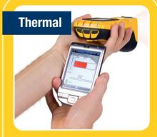
The Termatrac T31 remote thermal sensor with built-in laser pointer shows changes in surface temperature; a common sign of termite infestation.
