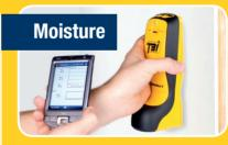
The moisture sensor confirms that conditions need further investigation. The moisture component enables the Geelong Pest Control technician to easily identify areas of excess moisture as a possible risk area for termites. The moisture sensor is so sensitive it can even pinpoint rising damp.
